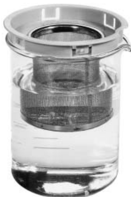
Fig 3. Mesh basket supported in a 600ml glass beaker during pre-soaking and ultrasonication. The plastic supporting ring is provided with the basket and the glass beaker fits the ultrasonic unit supporting ring.
