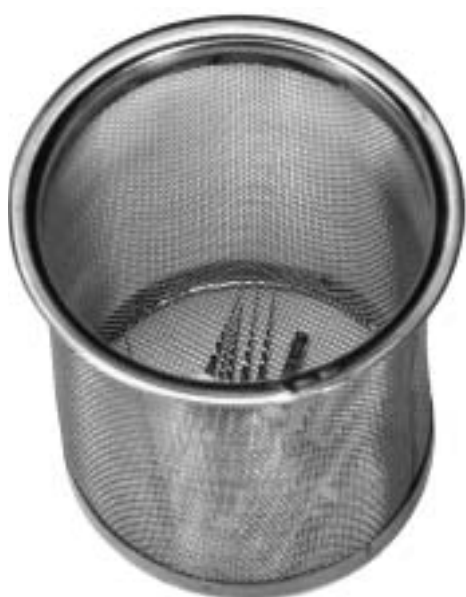
Fig 2. Small metal mesh basket used to support the files during pre-soaking and ultrasonication.
