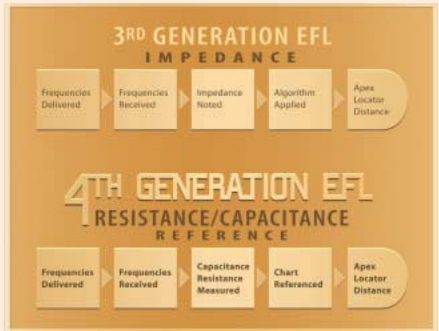
FIGURE 5 —The graphic shows the technologic difference between the operation of third and fourth generation foramenal locators.
