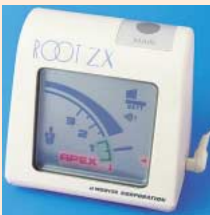
FIGURE 7 —The Root ZX® is a fully automatic, self-calibrating root canal foramen locator.
